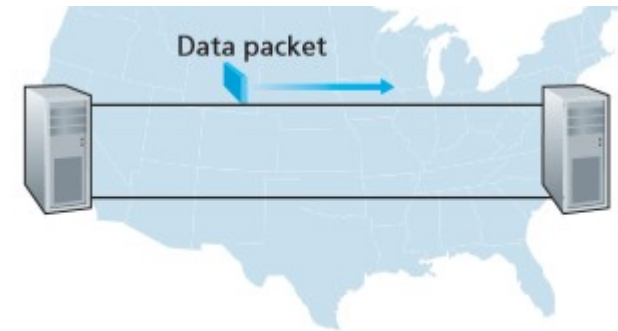
a. A stop-and-wait protocol in operation
