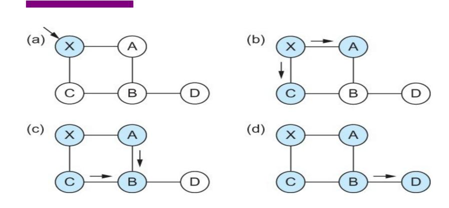
Flooding of link-state packets. (a) LSP arrives at node X; (b) X floods LSP to A and C; (c) A and C flood LSP to B (but not X); (d) flooding is complete
