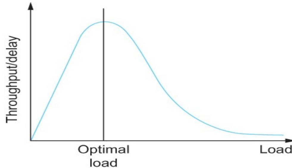
Ratio of throughput to delay as a function of load
