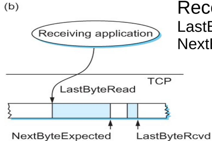
Relationship between TCP send buffer (a) and receive buffer (b).
