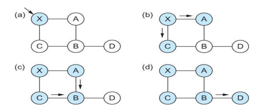
Flooding of link-state packets. (a) LSP arrives at node X; (b) X floods LSP to A and C; (c) A and C flood LSP to B (but not X); (d) flooding is complete
