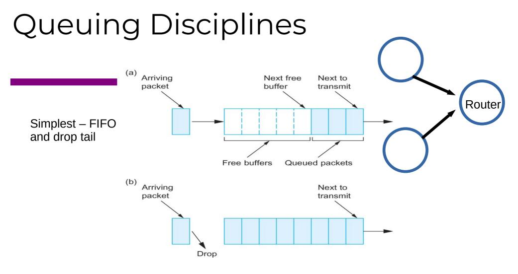
(a) FIFO queuing; (b) tail drop at a FIFO queue.
