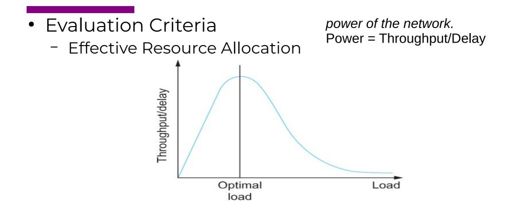
Ratio of throughput to delay as a function of load
